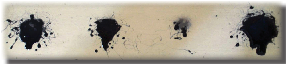
Spray pattern using commercial grade lubricant. Traditional asphaltic lubricants cause spray nozzles to clog, leading to poor application of the lubricant and the creation of damaging hot spots on gears.
